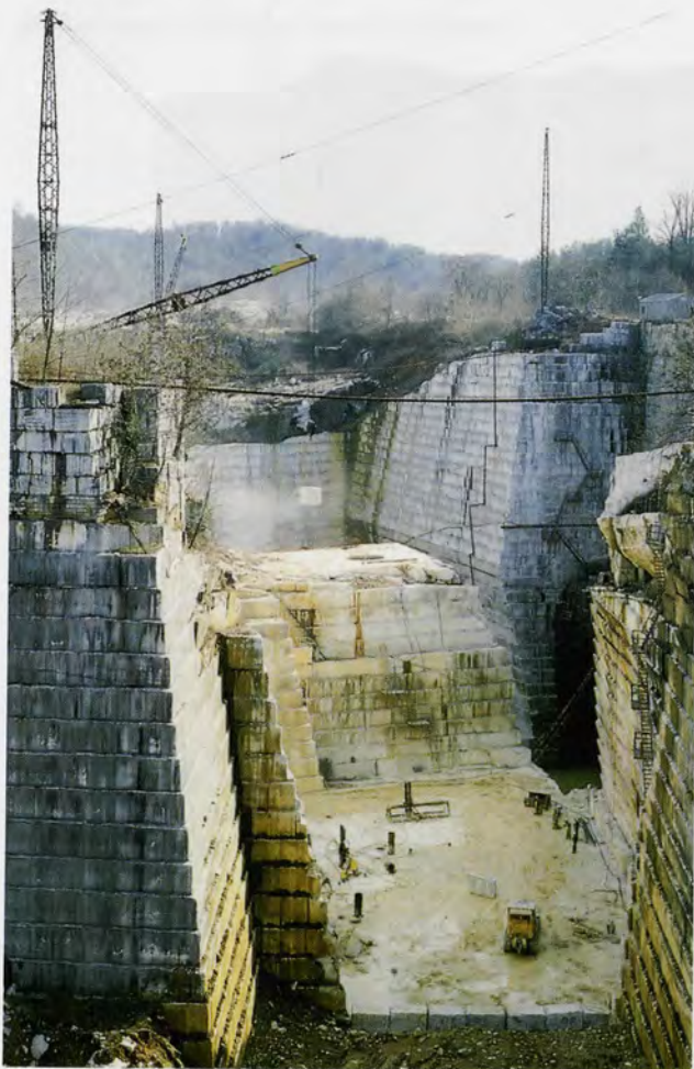
A 1970s photo of a Georgia Marble quarry. This is the largest open pit marble quarry in the world. Until the 1980s, derricks lifted the twenty ton blocks from the quarry. Today, the blocks are carried out of the quarry by road to the plant.
