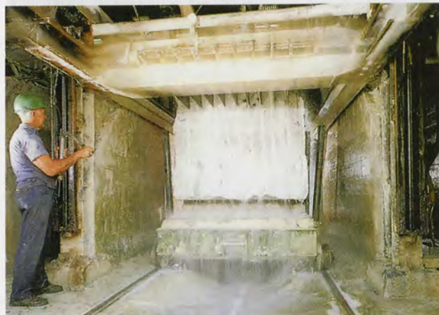
Huge gang saws cut the block into slabs.
