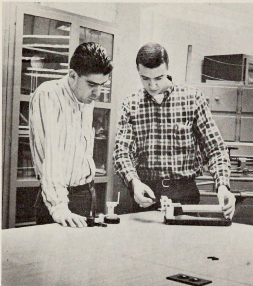
The Presley ratio indicates cotton tensile strength.
