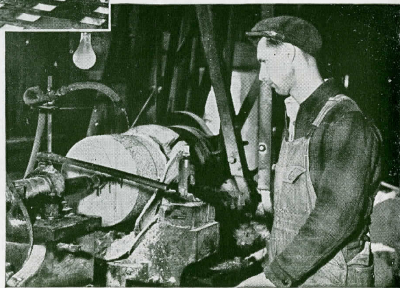
Urns, vases, small columns, balustrades, are turned on lathes
