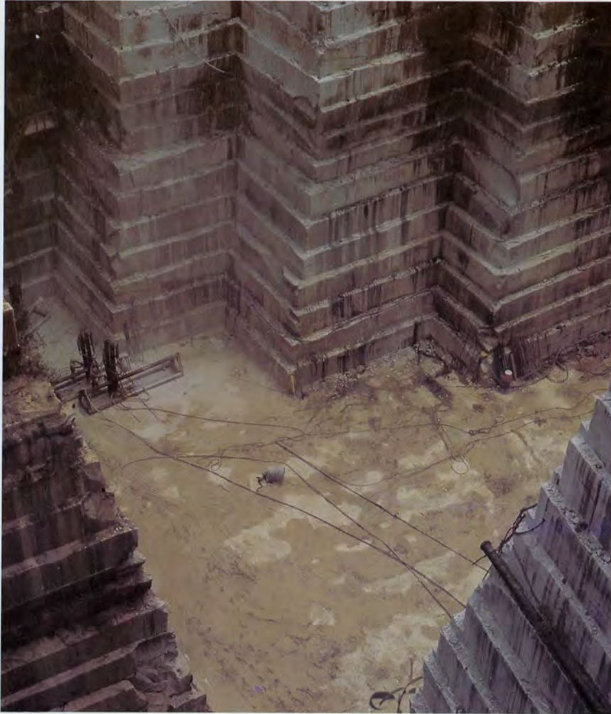
Workmen remove Georgia Marble from the bed of this man-made canyon, a small section of a quarry in North Georgia's Long Swamp Valley. Tiered walls of solid marble yet to be cut promise supplies for centuries to come.
