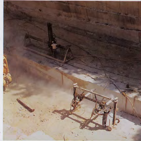
The quarry bar machine at upper left travels forward cutting narrow vertical channels through the solid marble bed. At lower right, a gadding machine cuts through the stone horizontally to release the block from the bed.
