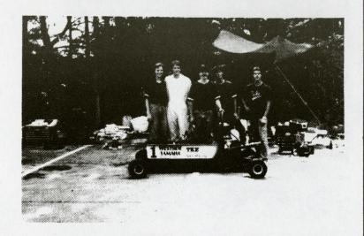
CHARACTERISTICS: Margay Wheels, Bridgestone Racing Slicks. Dual Rear Disc Brakes, Adjustable Camber Front Spindles, &075 Aluminum Axle, Yamaha YZ125 Engine
