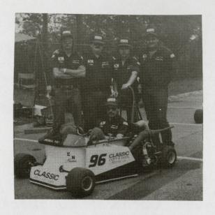
CHARACTERISTICS: 4 Foot Acid Dipped, Single Member Chrome-Moly Frame, Driver Ejected Quick Change Fuel Cell, Mechanical Full Pump, Quick Release Body Panels, Adjustable Cast/Chamber Front Spindles, Cylinder Temperature Gauge, Bridges Racing Slicks, Dual Rear Disc Brakes, Rotax 175 Air Cooled Engine
