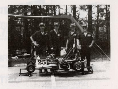
CHARACTERISITICS: 125cc Liquid Cooled Rotax Engine, 4-Wheel Disc Brakes and More Trick Stuff
