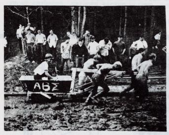
The formula for a bathtub racer is simple: take any cast iron, rolled rim bathtub four feet in length, acid-dip or grind it to the minimum 140 pounds, mount it on a lightweight frame, attach a 175 cc motorcycle engine, devise a steering system, install dependable brakes, and mount the whole thing on low profile Go-Kart racing slicks and you're in business.
